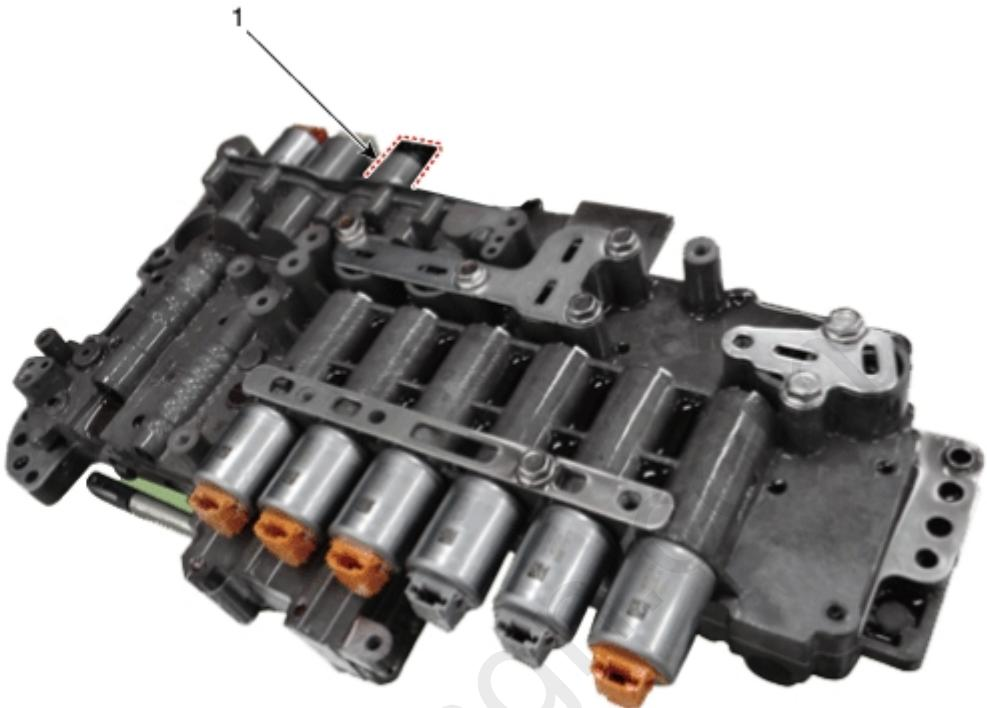
1. SS-A solenoid valve (ON/OFF)
